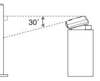
Keystone distortion can be corrected within a maximum vertical angle of approximately 30°.
