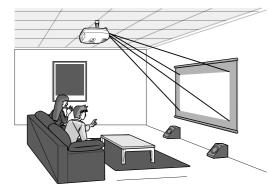
When suspending the projector from a ceiling, change the configuration menu settings.
