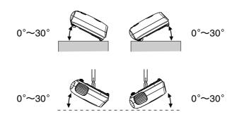
If you set the projector higher than 30°, it could damage the projector and cause an accident.
